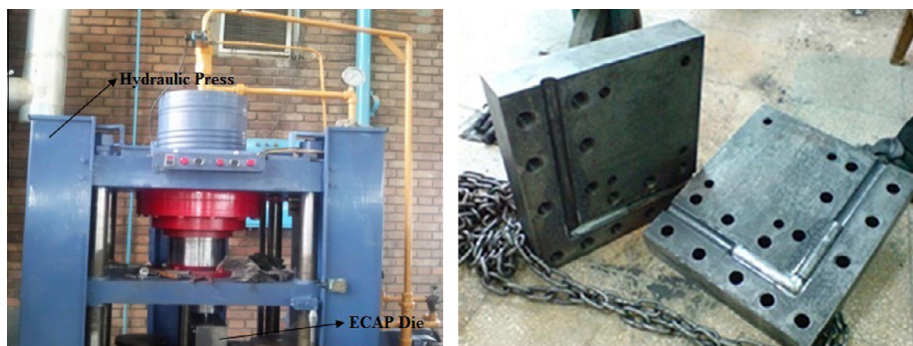
Fig. 1. Hydraulic press set-up and ECAP die with \varphi = 90^\circ and \psi \approx 15^\circ .
