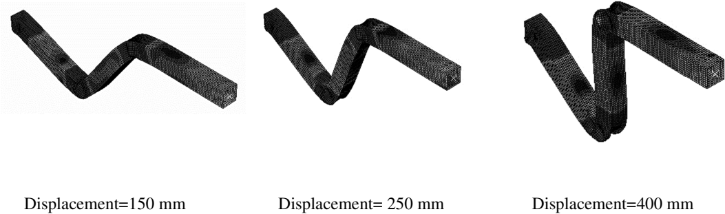
Fig12. shape of deformation of the S-rail with geometries of R=550\text{ mm} , q=25 , W=50\text{ mm} and t=2\text{ mm} at end displacement of 150, 250 and 400 mm.
