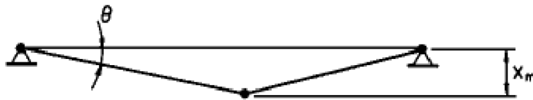
Figure 10. Relative support rotation in beam members [18]
