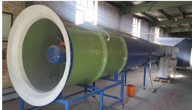
Figure 7. Schematic view of open-circuit wind tunnel
