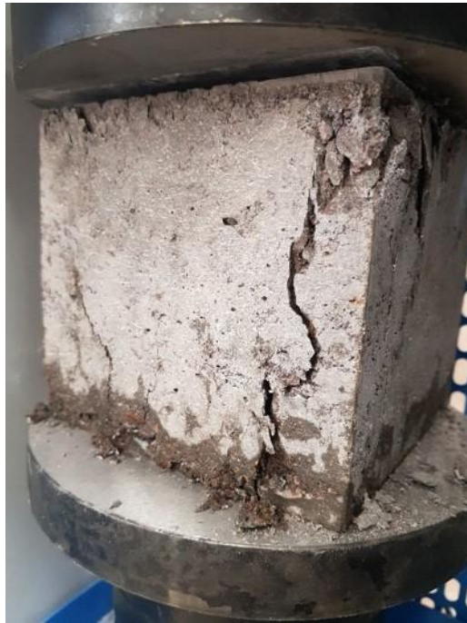
Figure 3. Failure of a concrete specimen
