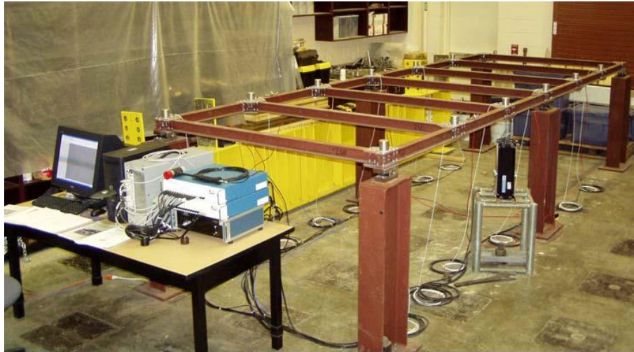
Figure 9: Two-Span Steel Grid benchmark [26]
