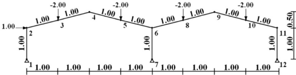
Figure 5. The geometry and loading conditions of Example 3.
