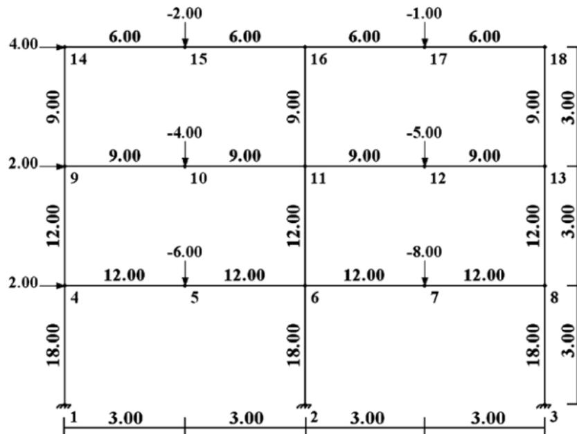
Figure 1. The geometry and loading conditions of example 1.
