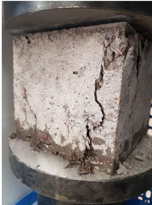
Figure 3. Failure of a concrete specimen
